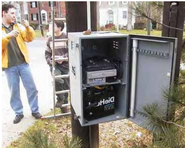
Figure 3. Portable Archival Traffic History (PATH) video system.
