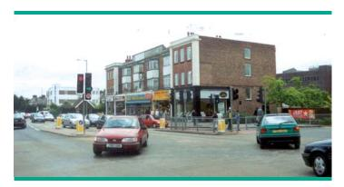
If the number of right-turners exceeds the number that can clear the junction in gaps, or during the intergreen, special provision will be probably be required. Note that if right-turners are left in front of the stop line after a change to another stage, not only will the driver feel in a vulnerable position but the presence of the vehicle may obstruct pedestrians wishing to cross.
