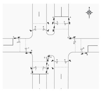
The only exception is at a junction where there is no rightturn from the approach losing right-of-way, the westbound approach in the diagram. The southbound approach will have a three-light primary and a secondary, which is always placed beyond the junction, with an additional right-turn arrow illuminated during Stage 2, see Diagram 4, Part 4. If the right-turn, from phase C, is still thought to be a problem the designer may consider a TRO to ban the movement.
